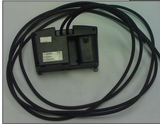
Right: Manometer and Air Flow Hood
