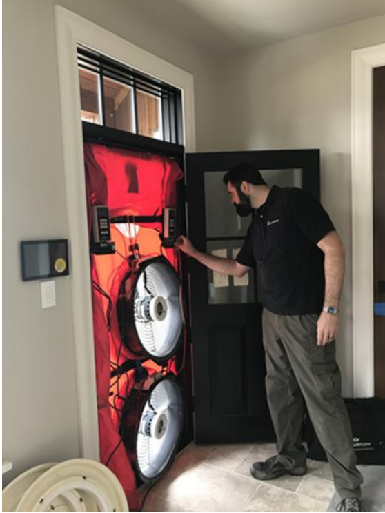
Left: "Blower Door" for air-tightness testing
